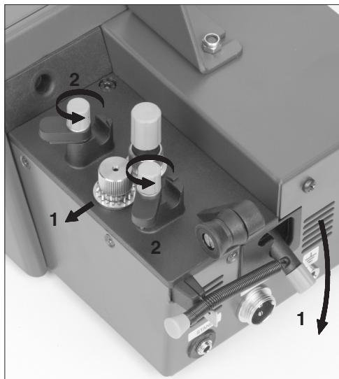
3. Place the tubes and guides set in the control unit. Tighten the screws.
