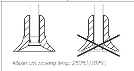
Insert the needle with the appropriate cup for a correct suction process.
