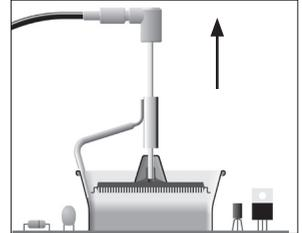
The component lifts off automatically when the solder melts.
